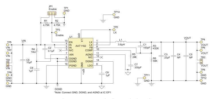
Figure 2: AAT1162 Evaluation Board Schematic.
