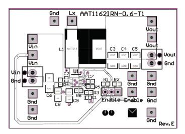
Figure 3: AAT1162 Evaluation Board Component Side Layout.
