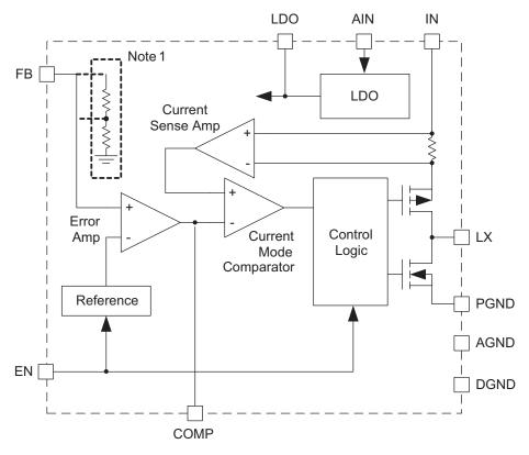
Note 1: For fixed output voltage versions, FB is connected to the error amplifier through the resistive voltage divider shown.
