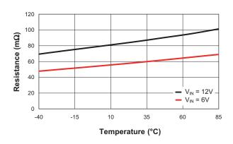
P-Channel  $R_{DS(ON)}$  vs. Temperature  $(V_{IN} = 6V)$
