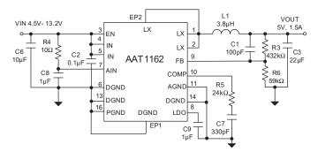
Figure 1: Typical Application Circuit.
